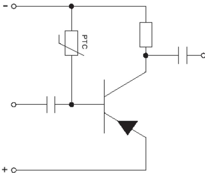
Fig.20 Temperature compensation of transistor
