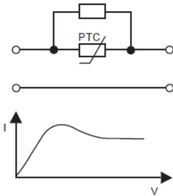
Fig.15 Current stabilization
