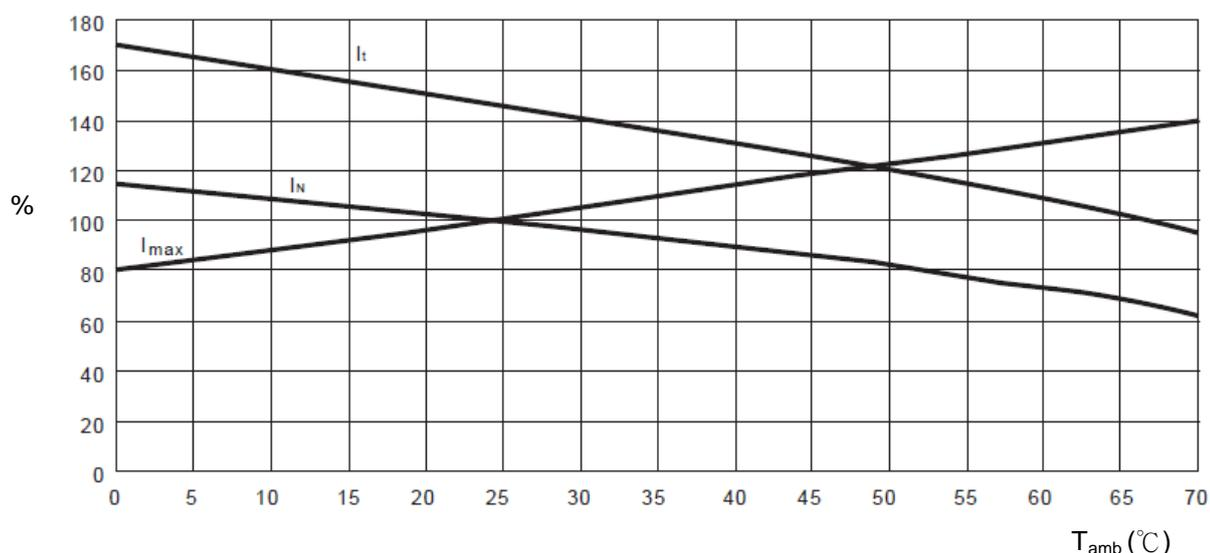
Fig. 12 Temperature V.S Current Curve
