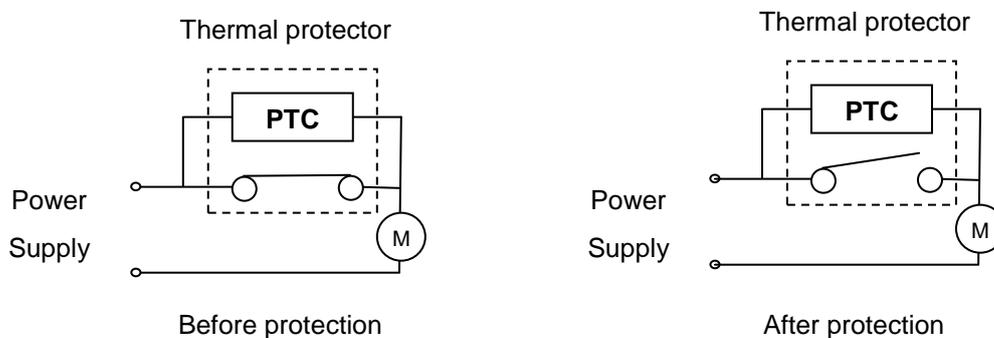
Fig. 23 Thermal protection
