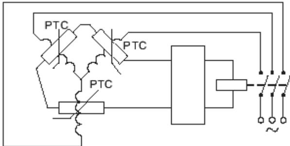
Fig.18 Temperature protection of electric motors
